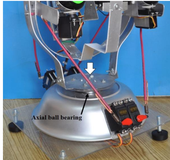
Figure 3. Implementation of the vertebral support of the NC. The atlas body module is on the upper cup of an axial ball bearing and the lower cup forms part of the scapular girdle module.
